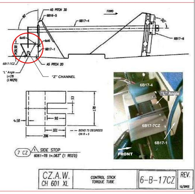
Parts needed: 1 Torque Tube Stop
